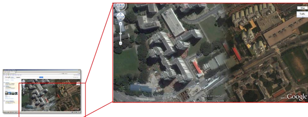
Figure 6: Singapore location, Google Earth, example of a photogrammetric parallax error of satellite imaging rendering. (accessed 16 July 2011).
