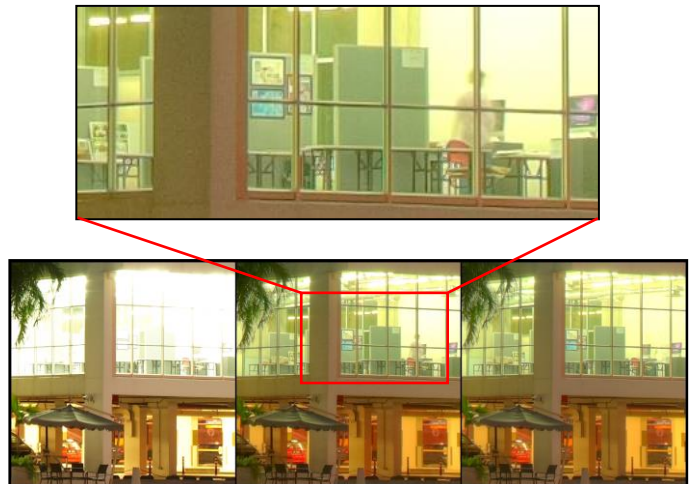
Figure 9. Magnified Lakeside Night Scene of Fig. 5(a), Fig. 5(b), Fig. 5(c) to observe the extended dynamic range and the noise appearance.
